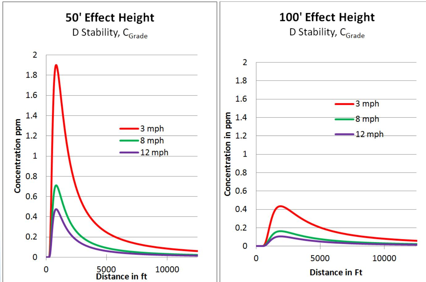
Concentrations Profiles at Grade for Two Different Elevation Releases, 50 ft and 100 ft
