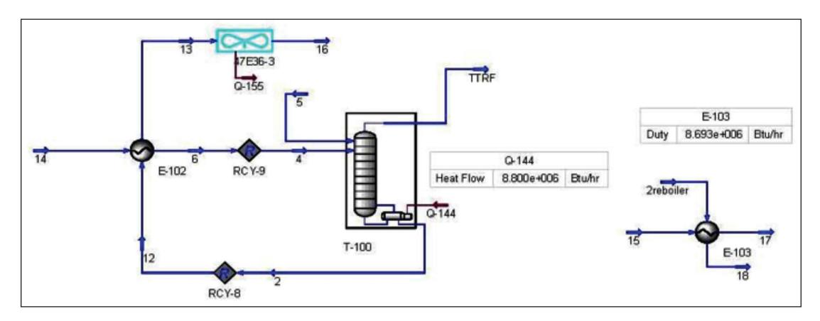
**Figure 1:** Example of a simulation for a column with loss of cooling and top-tower reflux failure with a reduced duty calculation performed.
