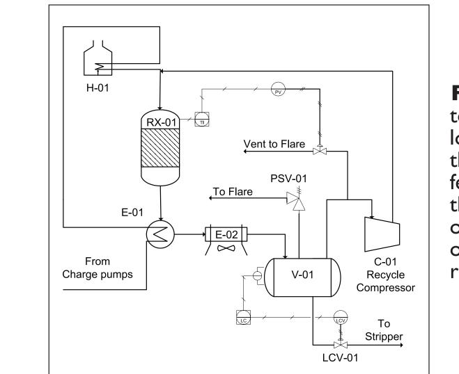
**Figure 4:** During an upset event due to the loss of the compressor, the relief load is not expected to be any larger as
