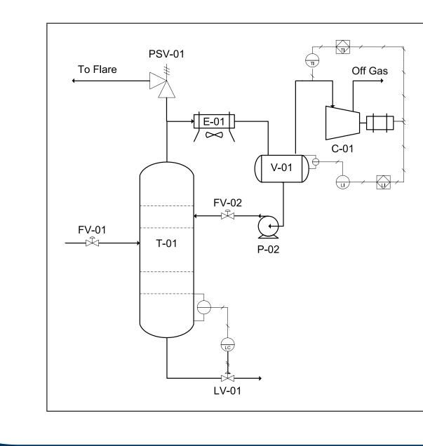
**Figure 5:** During a partial loss of cooling in E-01, the TI on the suction to C-01 may trip the motor to shutdown due to a high temperature reading. Due to the loss of the compressor, the credit for partial cooling cannot be taken as the vapor would accumulate and vapor lock the overhead condenser; thus, the partial loss of cooling would result in a completely blocked overhead outlet.
